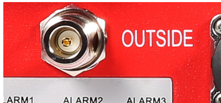
A1 — N-type Female for OUTSIDE cable and antenna
